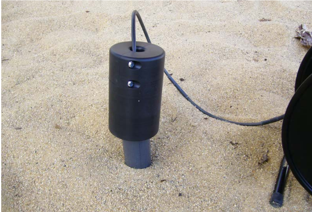
Fig. 5.2.2: Application of the cable guard
