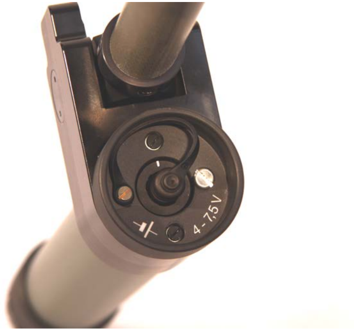
Fig. 4.6.1: Connection for external battery compartment
