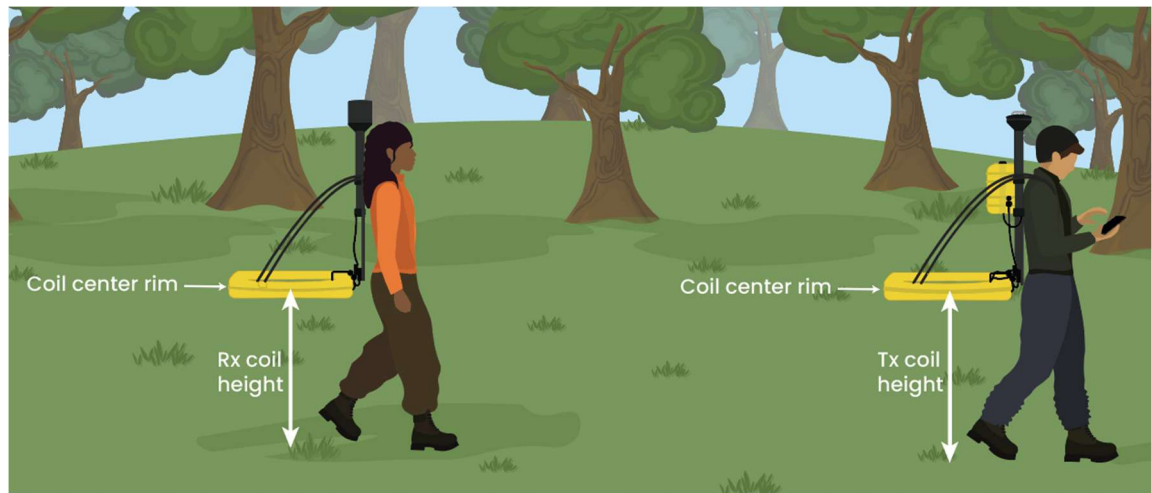
Figure 21: Depiction of proper coil height measurement
