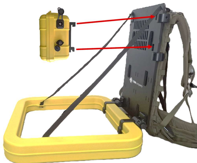
Figure 17: How to mount the TEM2Go unit onto the transmitter backpack.
