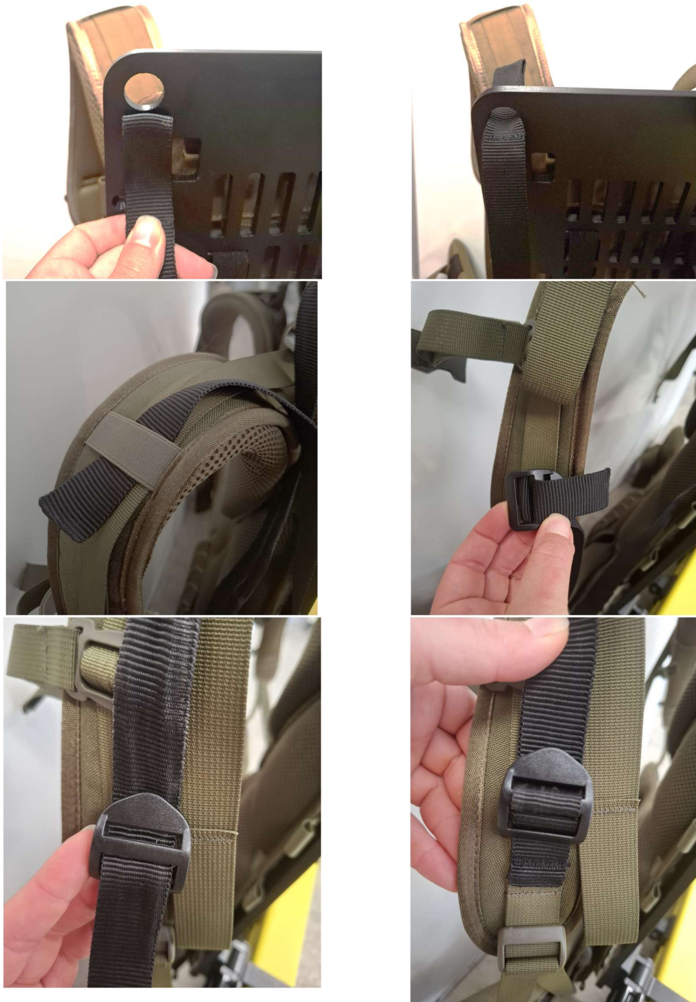
Figure 13: Detailed steps on how to secure the straps of the coil to the backpack.
