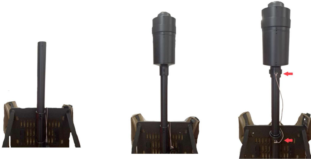
Figure 14: Mounting the Rx unit on the receiver backpack. Insert the pole in the bracket (left), add the Rx unit on top (middle) and secure everything with the provided clips (right).
