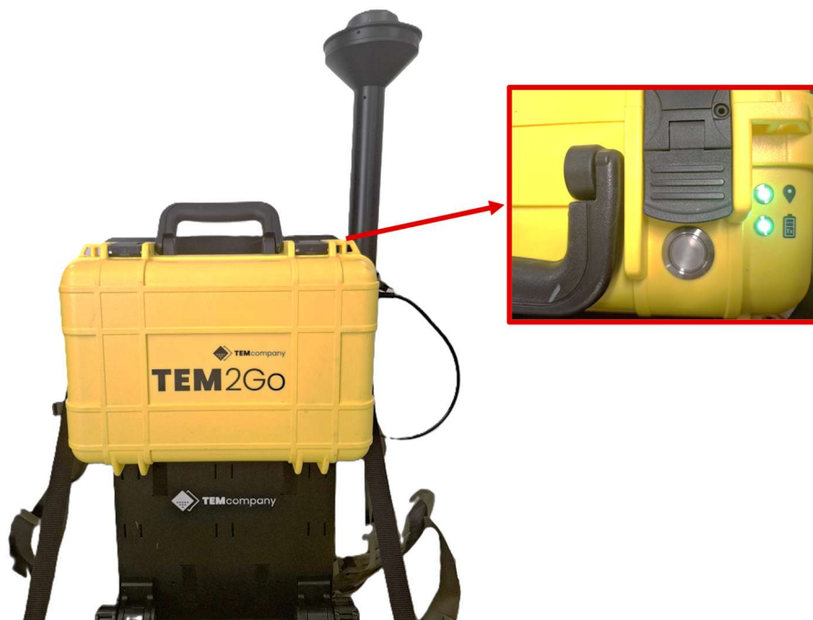
Figure 19: Once the Tx mast is connected to the unit the LED indicator will light up when it's receiving signal
