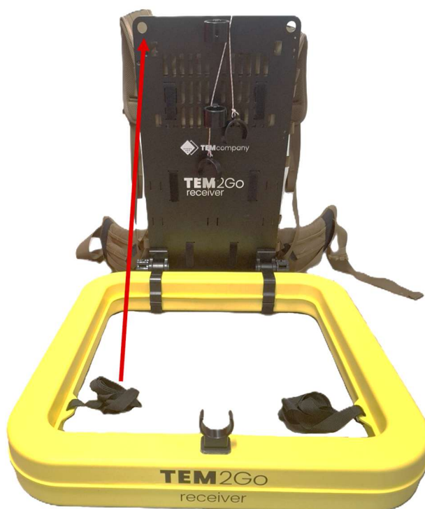
Figure 12: Assembled receiver backpack and coil. Last steps include securing the straps to the backpack.
