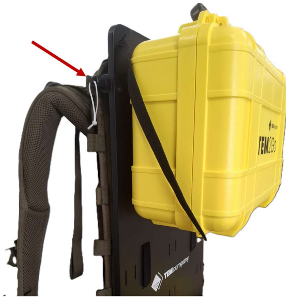
Figure 22: Remove safety pin to dismount the TEM2Go unit from the backpack.
