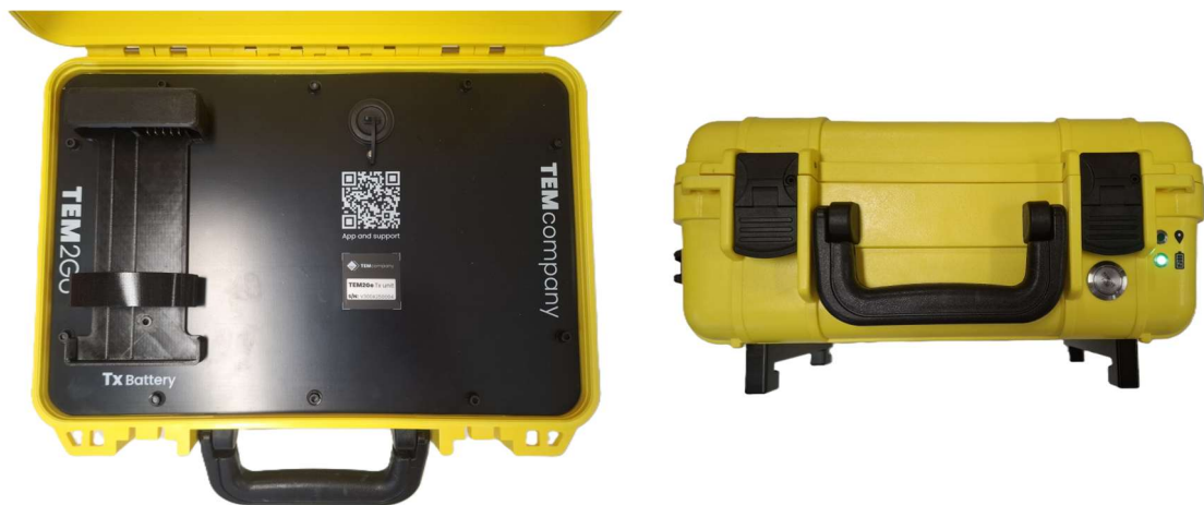
Figure 9: Battery slot of the TEM2Go unit (left) and LED light indicating the unit has been powered on successfully (right).
