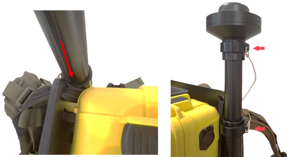
Figure 18: Insert (left) and secure (right) the Tx mast onto the transmitter backpack.
