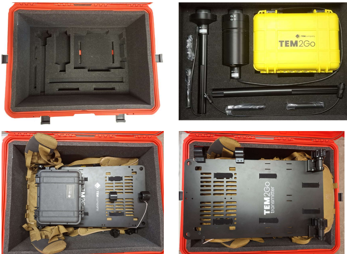
Figure 24: Packing components in the hard case. Start by packing the smaller components in the designated slots in the foam (up). Next pack the two backpack plates, with the battery charging suitcase located between them (down).
