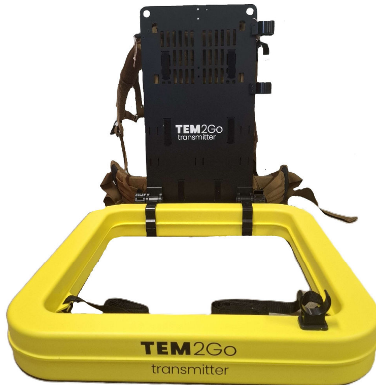
Figure 16: Assembled transmitter backpack and coil
