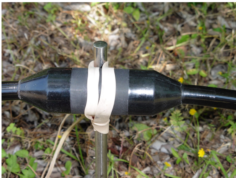
Figure 48: Graphite electrode, secured to the stake with a rubber band
