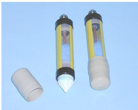
Figure 46: Non-polarizable electrodes, 6" x 1.25"
