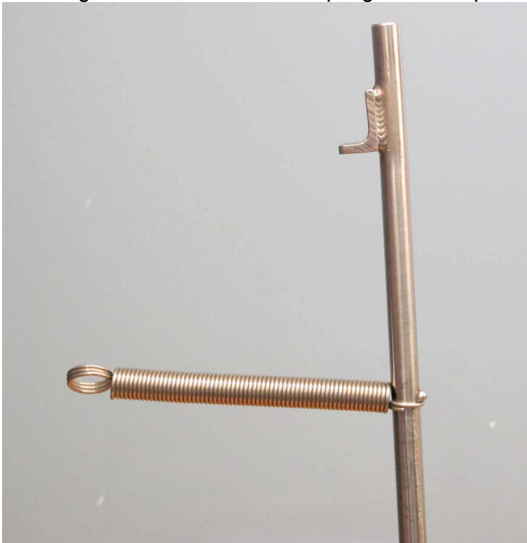
Figure 46: Push the spring to the stop knob
