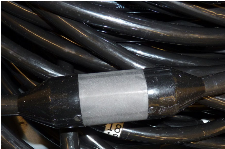
Figure 50: Graphite electrode molded onto a marine streamer
