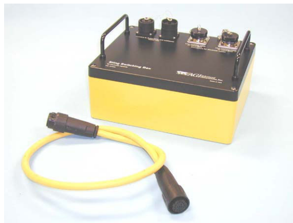
Figure 37: The switch box is available in 28, 56, 64, 84, and 112 electrode capability, and for both the SuperSting R8 and the SuperSting R1
