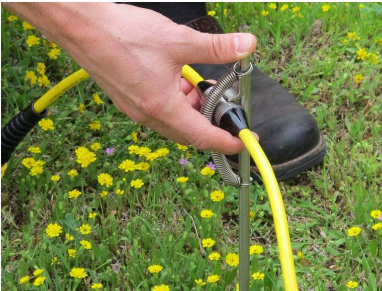
Figure 40: With two fingers, one on each side of the spring, grab the take-out and lift it up over the shelf.
