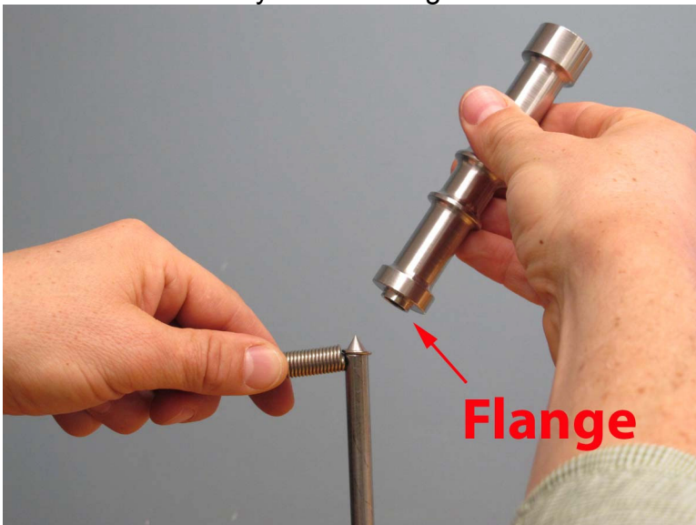
Figure 44: The flange side of the mounting tool faces the spring
