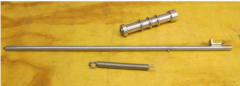
Figure 42: Spring (large loop to the left, small loop to the right), stake, and spring mounting tool
