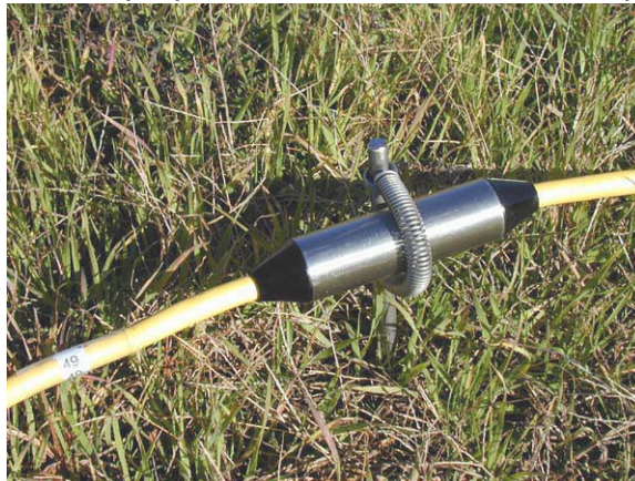
Figure 19: Attach the electrode switch to the stake by using the stainless steel spring
