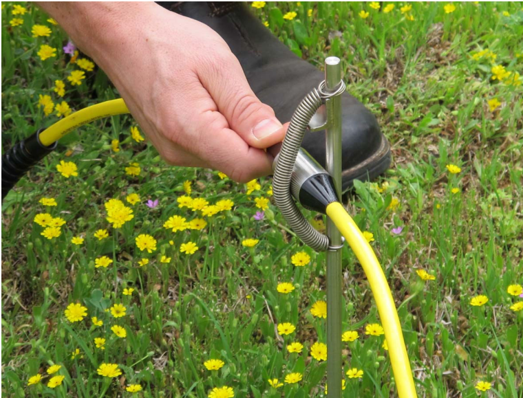
Figure 39: Slide the electrode take-out in under the spring and under the shelf.
