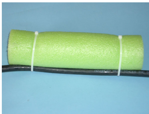
Figure 51: float tied to the cable
