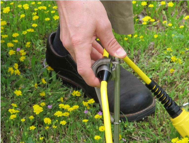
Figure 41: The take-out is in place, held firmly by the spring, creating a good mechanical and electrical connection.
