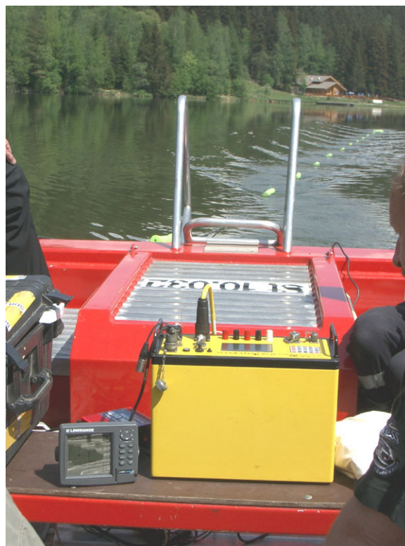
Figure 52: Starting the marine survey with floats attached to the electrode cable
