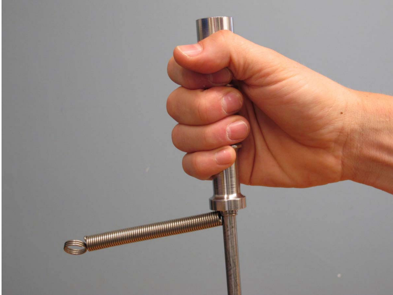
Figure 45: Using the mounting tool, push the spring down on the stake
