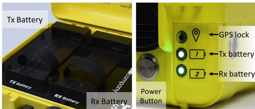
Figure 4. sTEM unit. Battery slots and battery LED lights when batteries are inserted.
