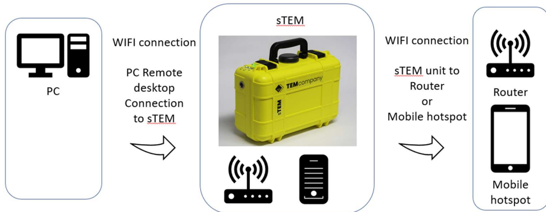
Figure 22. Flowchart for how to put sTEM unit online.
