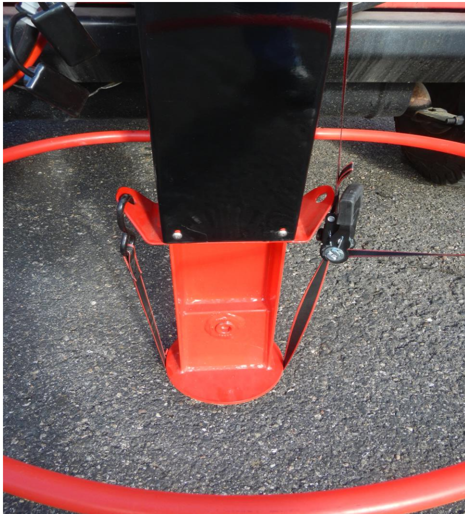
FIGURE 5 Shows Hammer held to the exact height necessary to put the 2" square tube into the standard 2" receiver
