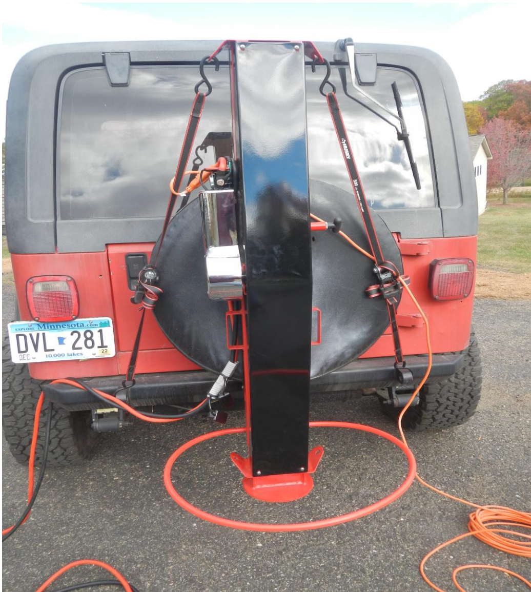
FIGURE 6 Always install Red Guard to keep everybody away from the hammer impact area.
