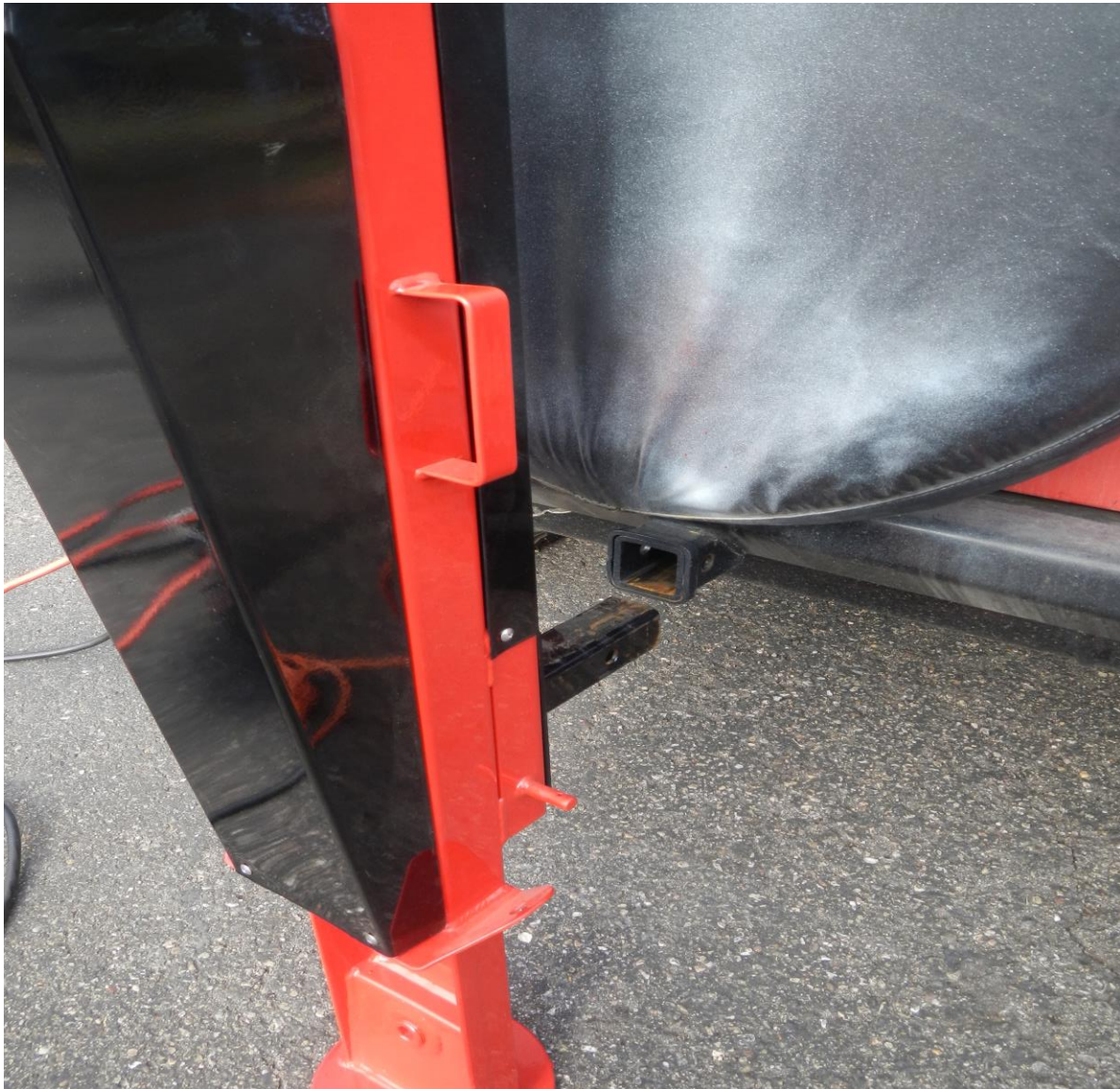
FIGURE 2 BB50 Trailer Height Adjustment Fixture
