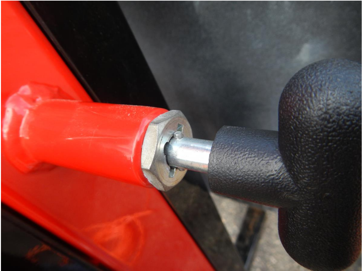
FIGURE 4 Safety Pin has cross pin to allow pin rotation and locked off
