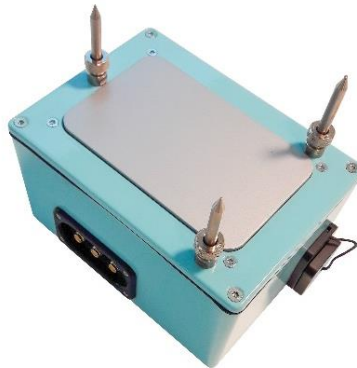
Figure 14. Mount long spikes for recordings on soft soils/grounds or whenever significant spike penetration is possible.
