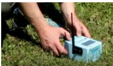
Figure 15. By alternatively pressing on the lowermost corners of the box and on the middle of the top edge above the display, set TROMINO® in a horizontal position.
