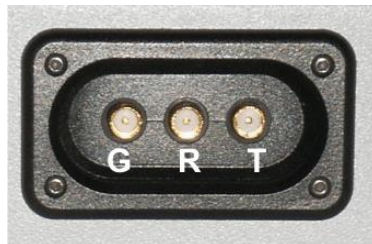
Figure 9. TROMINO ® right side connector panel. From left to right, G is the connector for the GPS antenna, R is the connector for the radio antenna (to be used also for the wireless trigger), T is the connector for the auxiliary channel (e.g., trigger cable). The GPS and radio antennas are not intended to work simultaneously.
