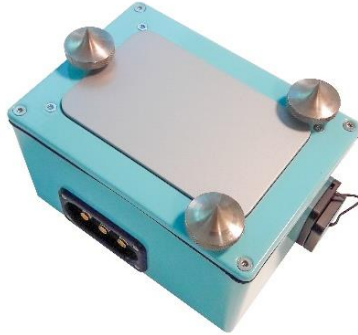
Figure 13. Mount the short spikes to perform acquisitions on solid rock, inside buildings and in all cases where the soil/ground is too stiff to allow significant penetration. Level the instrument by slightly rotating the spikes.
