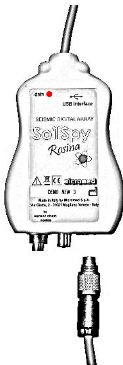
Figure 5. Connection between the SoilSpy head and the USB interface.
